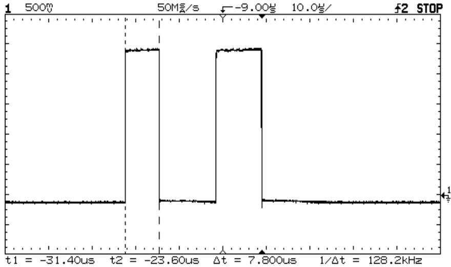
Pressing  $t_1$  and  $t_2$  softkeys simultaneously causes the time cursors to move together when the cursor knob is adjusted.
