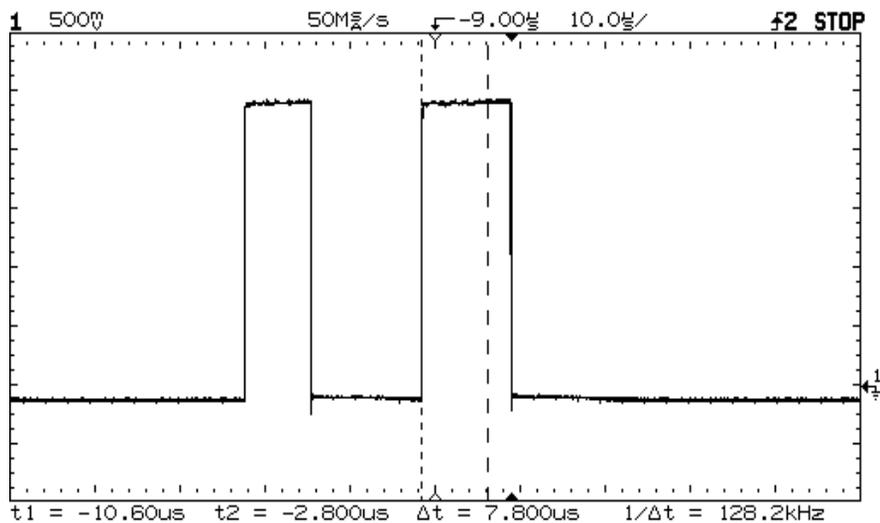
By moving the time cursors together, you can check for pulse width variations in a pulse train, as figures 2-15 and 2-16 show.
