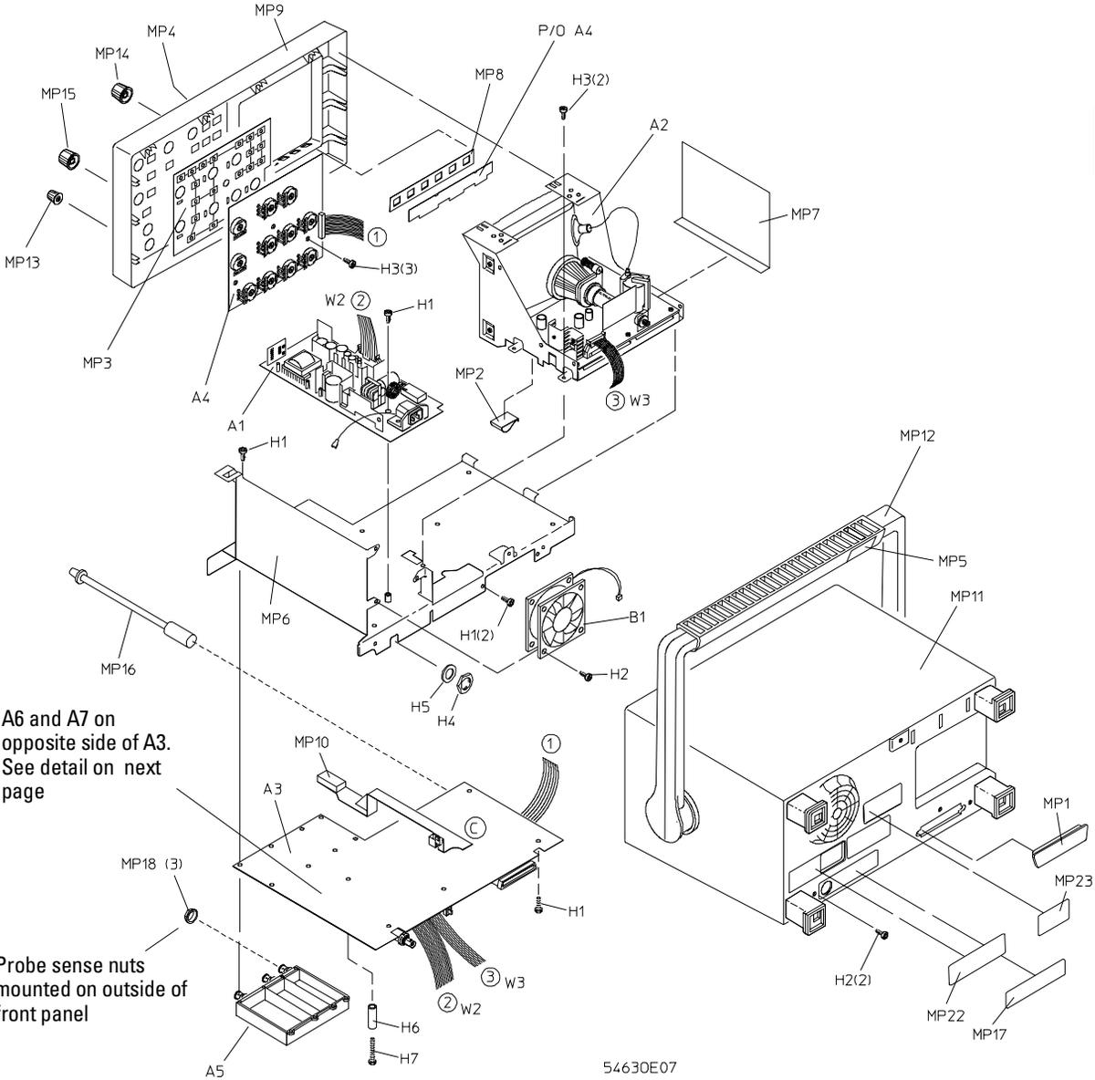
Exploded view of oscilloscope
