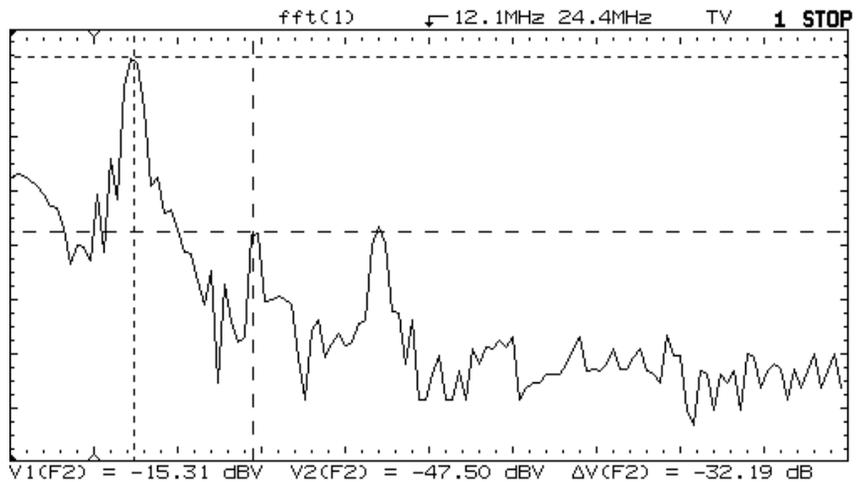
**The FFT function shows that the harmonic content of the color burst is more than 31 dB below the subcarrier**
