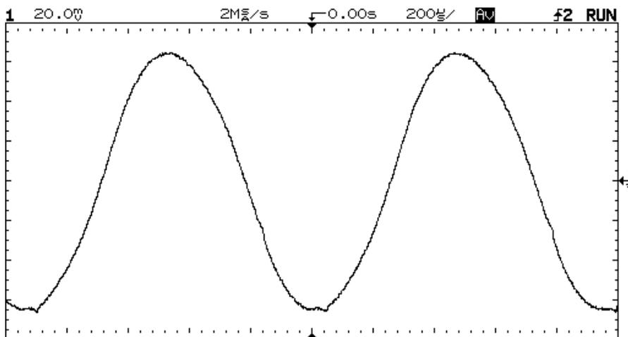
**On this waveform, 256 averages were used to reduce the noise**
