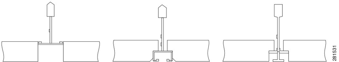
Figure 5 Adapter Clips Installed with Ceiling Grid Clips
