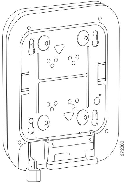
**Figure 2** Universal Bracket Installed on an Access Point
